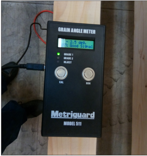
Figure 2. Device for measurement of grain angle.
