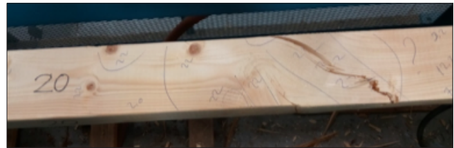
Figure 7. Large knot and associated grain distortions made up approximately 90% of the cross section of the deviant specimen.
