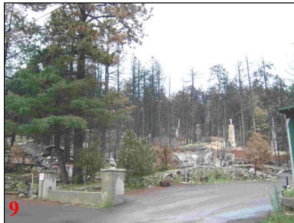
Photos 7,8,9—totally destroyed homes surrounded by unconsumed tree canopies indicate that lower intensity surface fires spread to the structures' surrounding areas.
