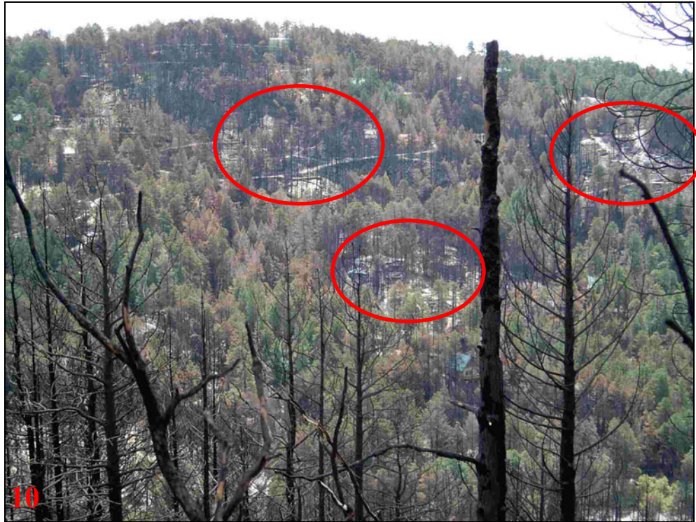
Photo 10 —patches of burned trees that are associated with multiple totally destroyed homes break the largely unconsumed forest canopy. The red ovals show 3 examples of this burn pattern.
