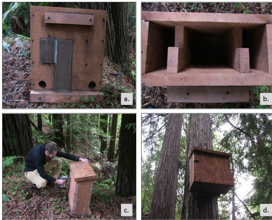
Figure 2. Humboldt marten box design for 16 boxes deployed at the Pecwan Creek study site in northwestern California, USA, between June and July 2013, including (a) tree-facing side of box including 2 lateral entrances; (b) box interior including 2 lateral access shafts and central inner chamber created by 2 baffles; (c) fully constructed box including attached roof; and (d) box mounted on a live tree.
