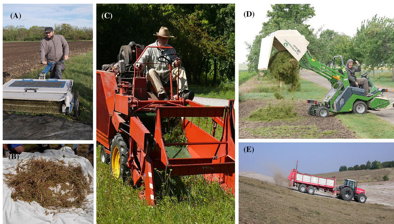
Figure 5 Seed-rich green hay harvested at a suitable donor site in Germany using equipment such as (A, B) a brush-type harvester that collects mature seeds and minimal vegetative material or (C) a plot harvester that produces threshed material. The seed-rich material should be transferred immediately to the receptor site and spread using equipment such as (D) a mower with a bucket spreader or (E) a manure spreader to restore species-rich near native grasslands and field margins. Photos: (A–D) A. Kirmer, (E) S. Mann.
