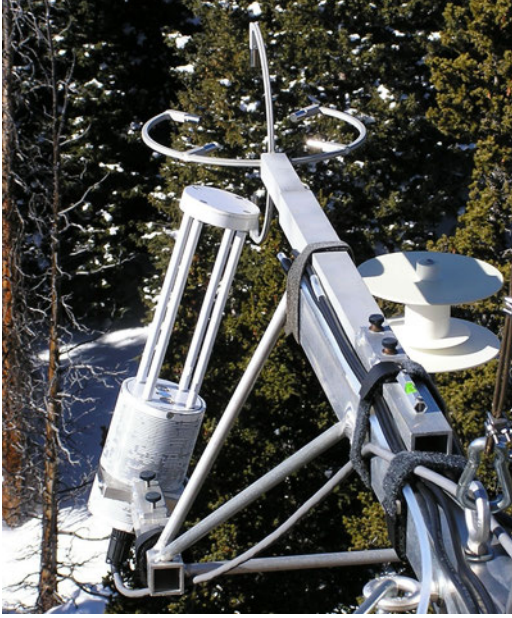
Fig. 2. The NOAA IRGA installed as part of the main GLEES eddy covariance system on 24 January 2006. The 2010 study was conducted on a replicate system mounted 2 m below.
