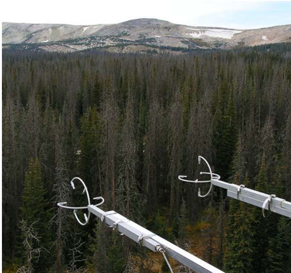
Fig. 1 The ATI 3Vx-probe GLEES experiment. The anemometer on the left is horizontally rotated around the u_c axis
