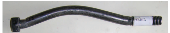
Fig. 19. (Color) Significant bolt bending as observed in the L/D = 10 tests.
