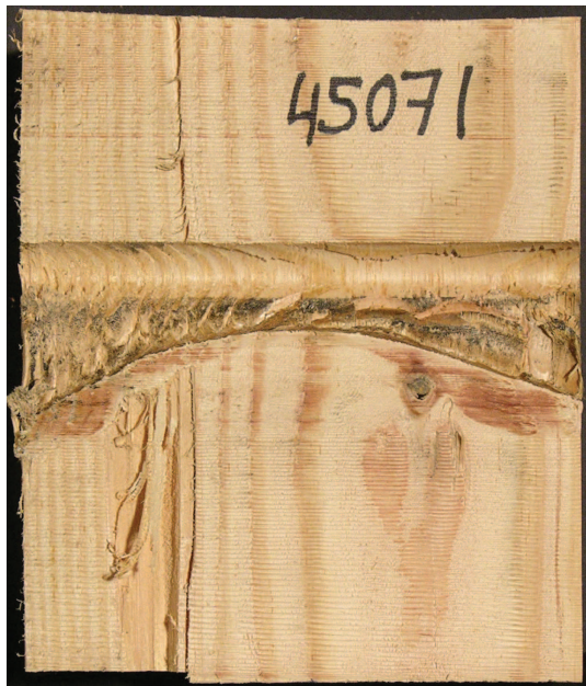
Fig. 17. (Color) Damaged bolt hole in 127-mm-thick wood ( L/D = 10 connector) due to bolt bending.
