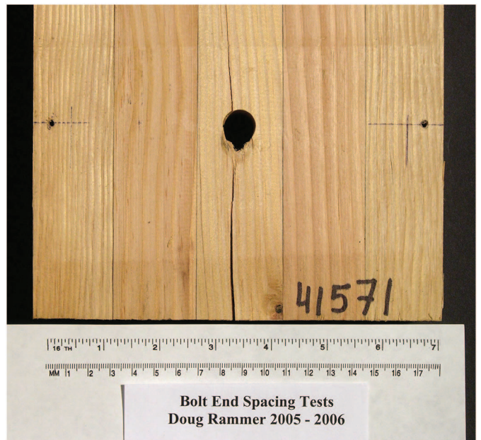
Fig. 20. (Color) Failed middle wood member of L = 38.1 mm ( L/D = 3 ) connector.
