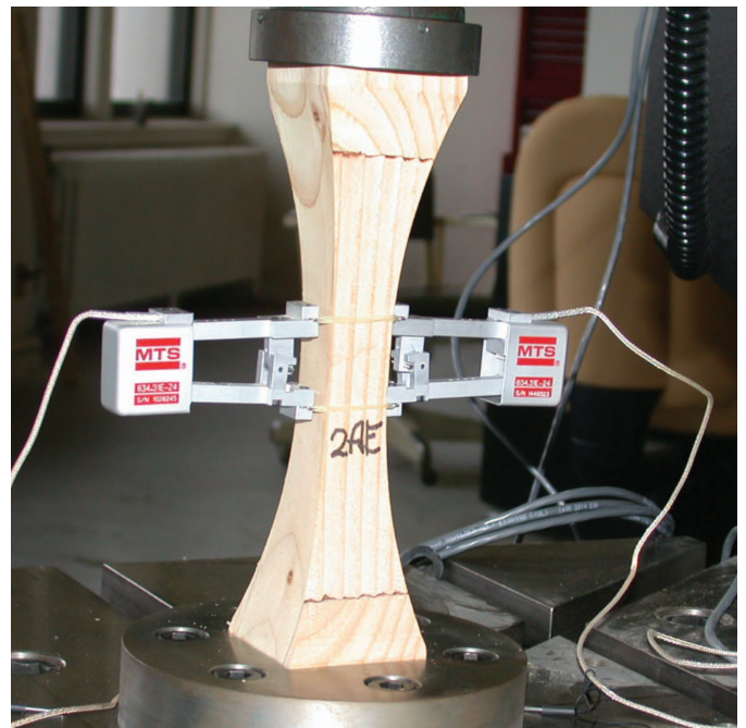
Fig. 6. (Color) Compression testing of Douglas-fir.
