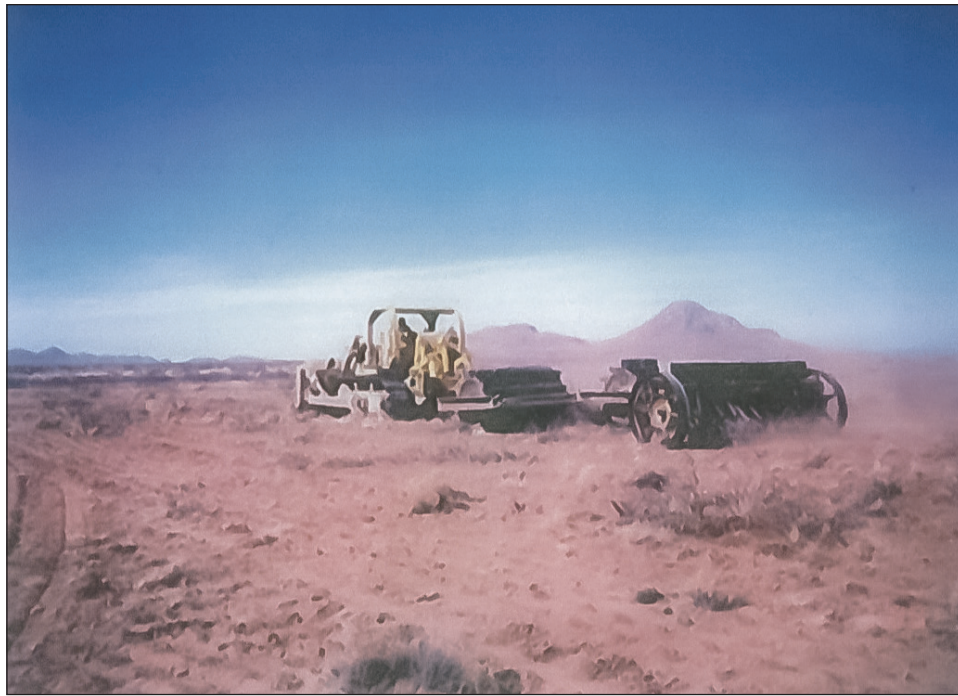
Figure 3 —Marden Brush Crusher and rangeland drill being pulled by a TD-25 at the George Wright pasture site.
