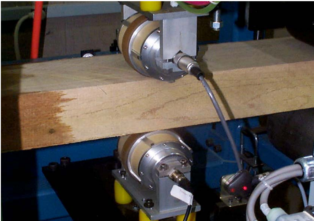
Figure 3. Close view of ultrasonic measurement through cant.
