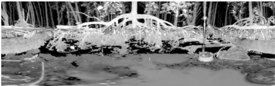
Fig. 3 An intensity image recorded by CBL. The brighter areas represent higher intensity returns, i.e., higher response in 905 nm, and vice versa
