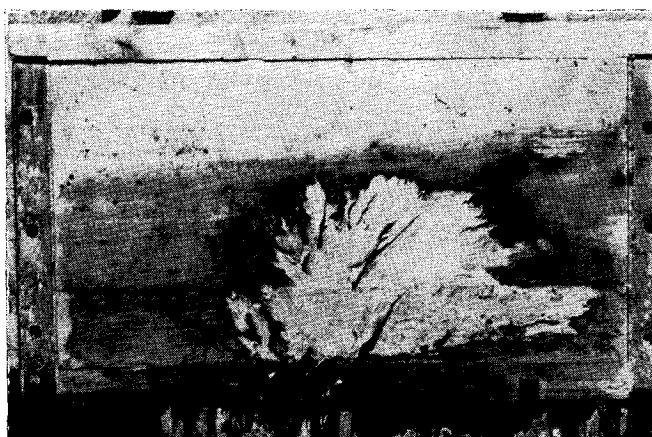
Fig. 2.—(Left) Black, wet rot. This rot, with a shell of softened wood, was common in many of the treated boxes in Panama. (Right) Mycelial fan of water-conducting rotter ( Poria incrassata ) growing upside of a dry box under tarpaulin cover. This fungus can rot boxes without rain-wetting, but is rarely encountered.
