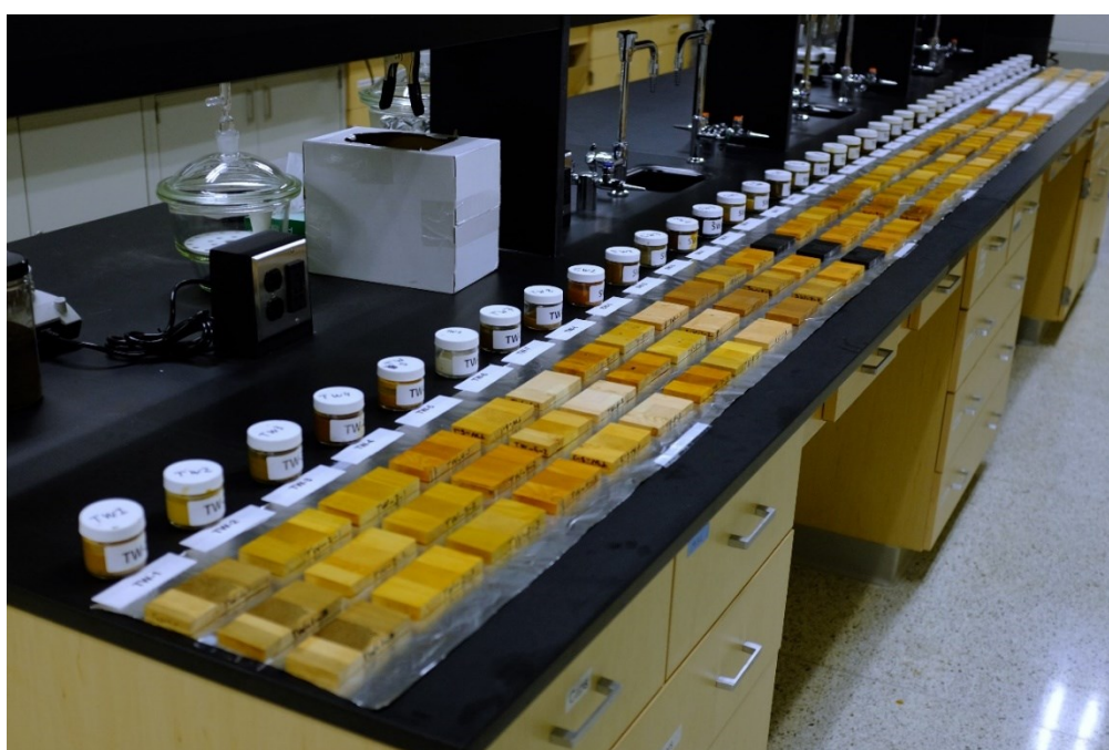
Figure 5. Image of coated small cross-laminated timber (CLT) samples.
