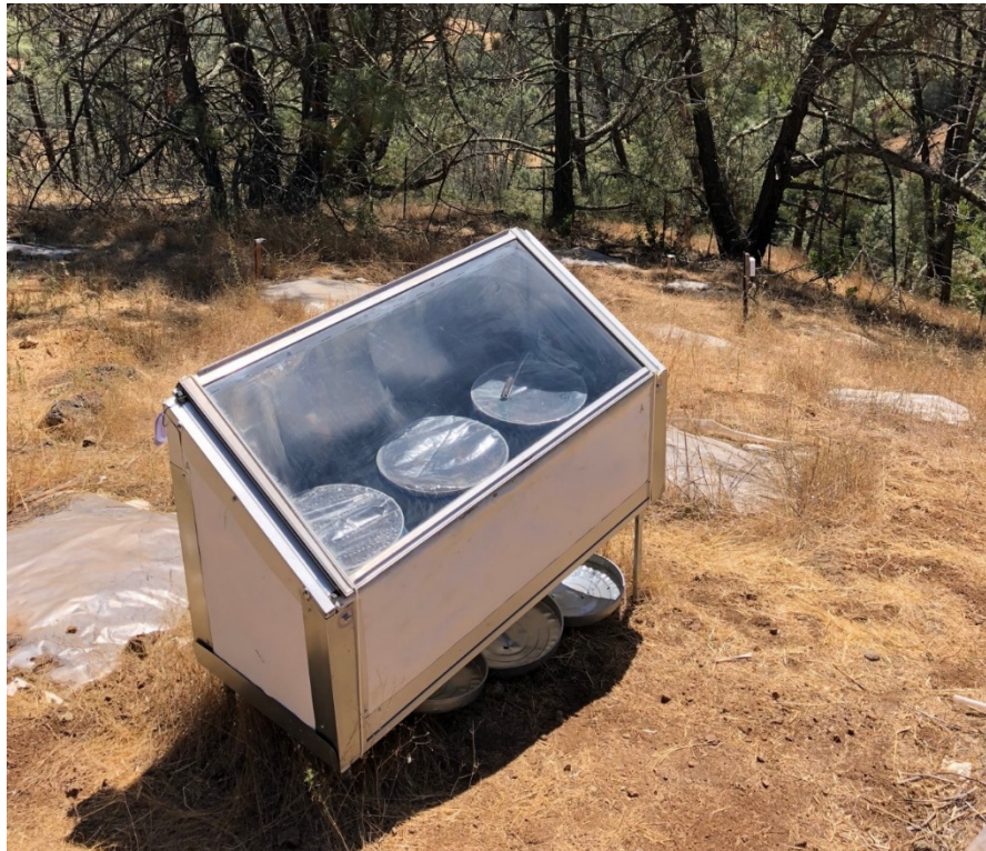
Figure 5. Solar oven used to heat treat soil from infested plant basins. Credit: Janell Hillman, SCVWD.
