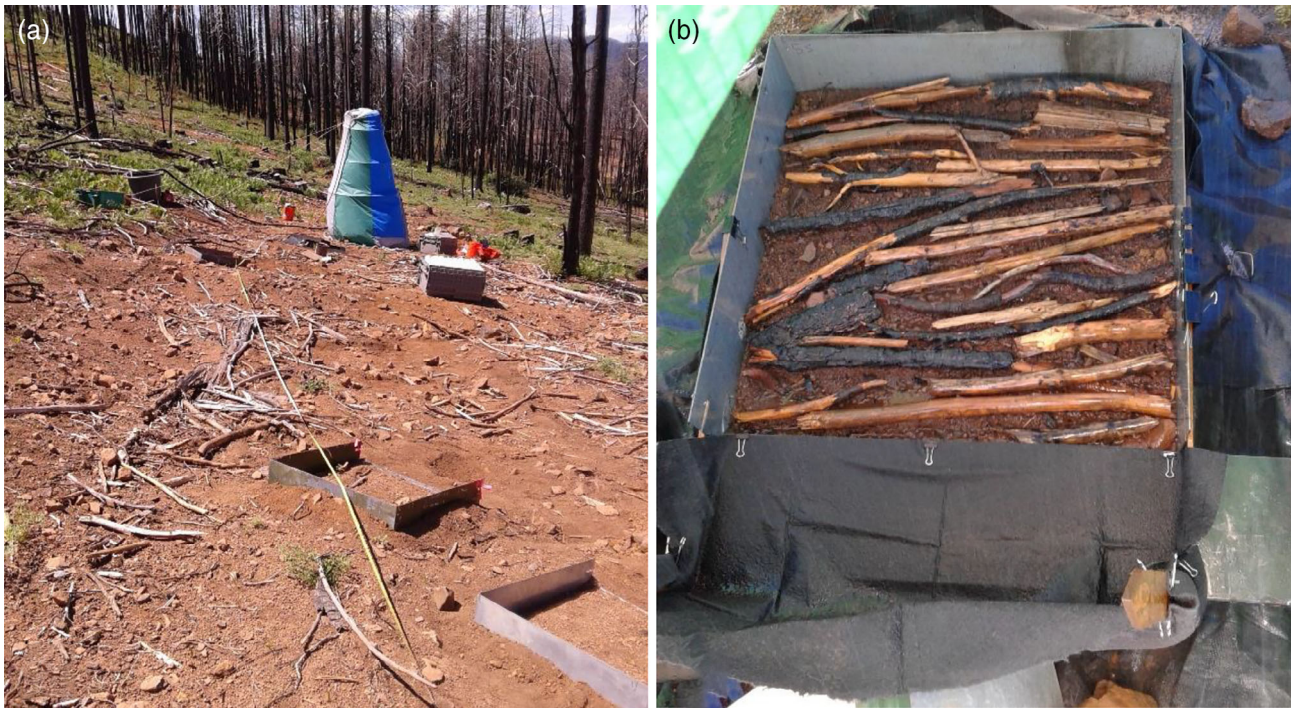
FIGURE 2 (a) Portable rainfall simulator assembled over one plot on the skid trail, with wind-shelter in place and (b) detail of a compacted and slash-covered plot and the splash-collecting system. The gutter is located 3 cm below the splash fabric
