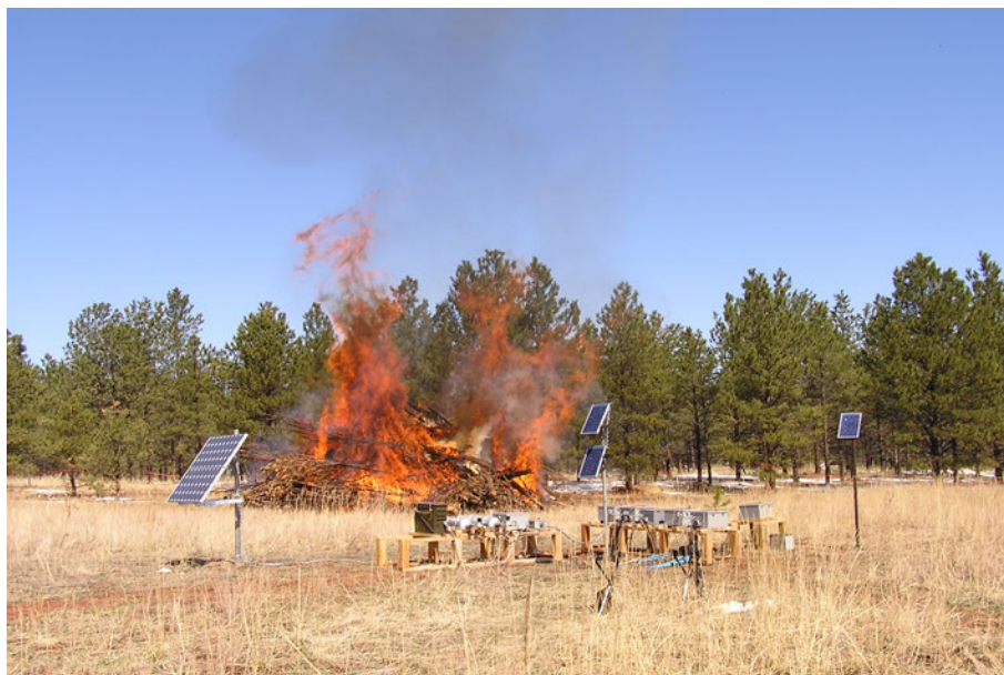
Figure 2. Layout of the data system and slash pile of the MEF 26 April 2004 experimental burn about 25 min after ignition. Image credit: John M. Frank.
