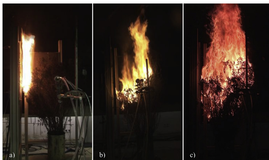
Fig. 6. Fire growth observed 30s after ignition for different values of \alpha : (a) low combustibility: \alpha = 0.10 \text{ kW s}^{-2} (fire test 4); (b) medium combustibility: \alpha = 0.22 \text{ kW s}^{-2} (fire test 14) and (c) high combustibility: \alpha = 0.52 \text{ kW s}^{-2} (fire test 15).
