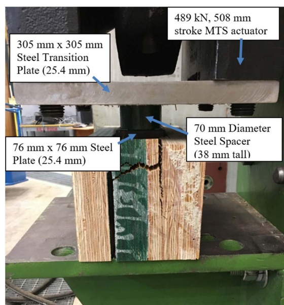
Fig. 1. Compression test setup for LVL block loaded in the X-direction. [Orientation according to ASTM D5456 (ASTM 2019).]
