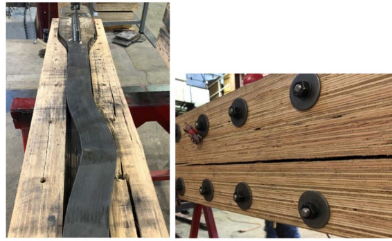
Fig. 16. Specimen 6 hysteresis for strain loading protocol and failure mode.
