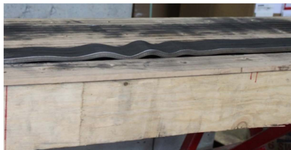
Fig. 14. Specimen 4 hysteresis for strain loading protocol and failure mode.
