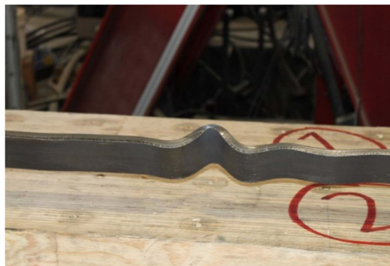
Fig. 13. Specimen 3 hysteresis for fatigue loading protocol and failure mode.
