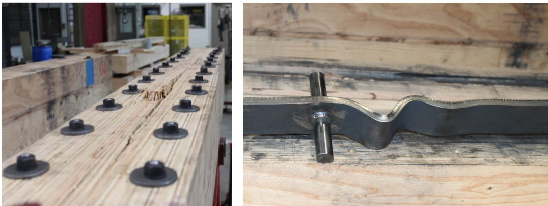
Fig. 12. Specimen 2 hysteresis for fatigue loading protocol and failure mode.
