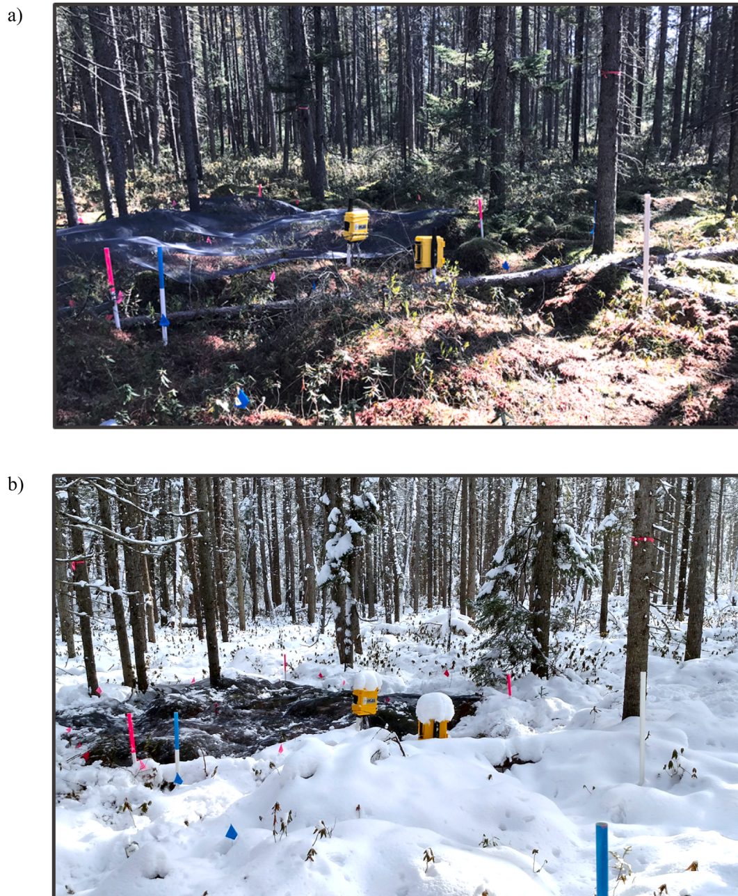
Fig. 2. Paired research plot during the autumn of experiment installation (a) and the winter of 2018 (b). In (a), the screening system for snow removal is visible on the snow removal plot (pink markers). The ambient snow cover plot does not have screening coving it and is delineated with blue markers. (For interpretation of the references to colour in this figure legend, the reader is referred to the web version of this article.)
