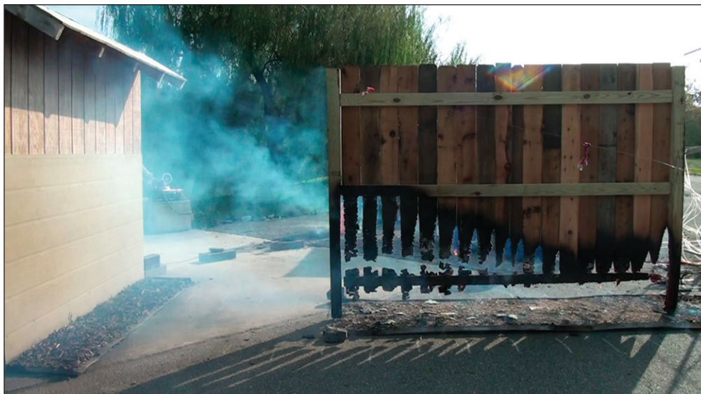
Figure 12 —Single western redcedar privacy fence in hardwood mulch at low wind speed ( 6 \text{ m second}^{-1} ).
