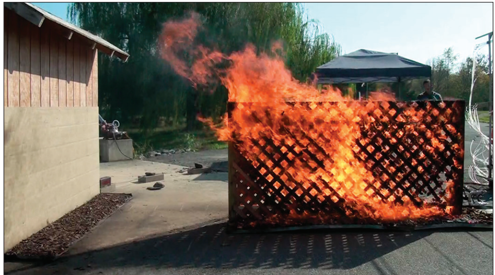
Figure 10 —Double redwood lattice fence in hardwood mulch at low wind speed ( 6 \text{ m second}^{-1} ).
