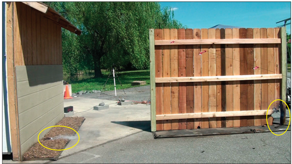
Figure 8 —Firebrand spotting for western redcedar privacy fence with high wind speed ( 14 \text{ m second}^{-1} ) and at 1.8 m separation distance from wall.
