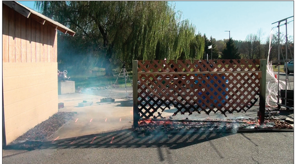
Figure 9 —Single redwood lattice fence in hardwood mulch at low wind speed ( 6 \text{ m second}^{-1} ).
