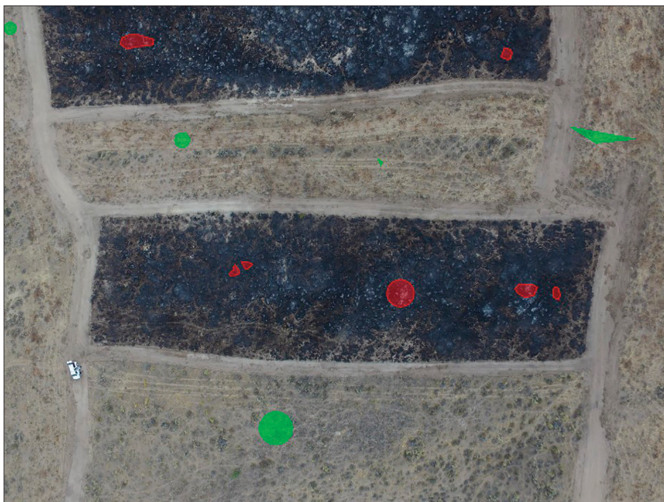
Figure 4 —Training pixel regions for training burn extent as denoted by the user using the Training Data Selector. Green polygons are unburned pixels, red polygons denote black ash pixels.
