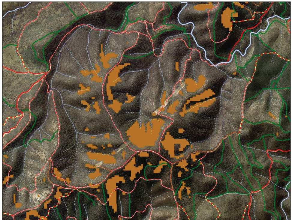
Figure 3 —Potential sources of debris flow within the Wombat Creek (Australian Capital Territory) burn; erosion source areas are indicated by brown shading.
