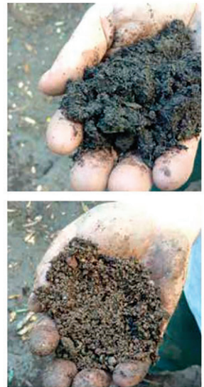
Eroded material from burned areas consists of ash, organics and mineral soil.
