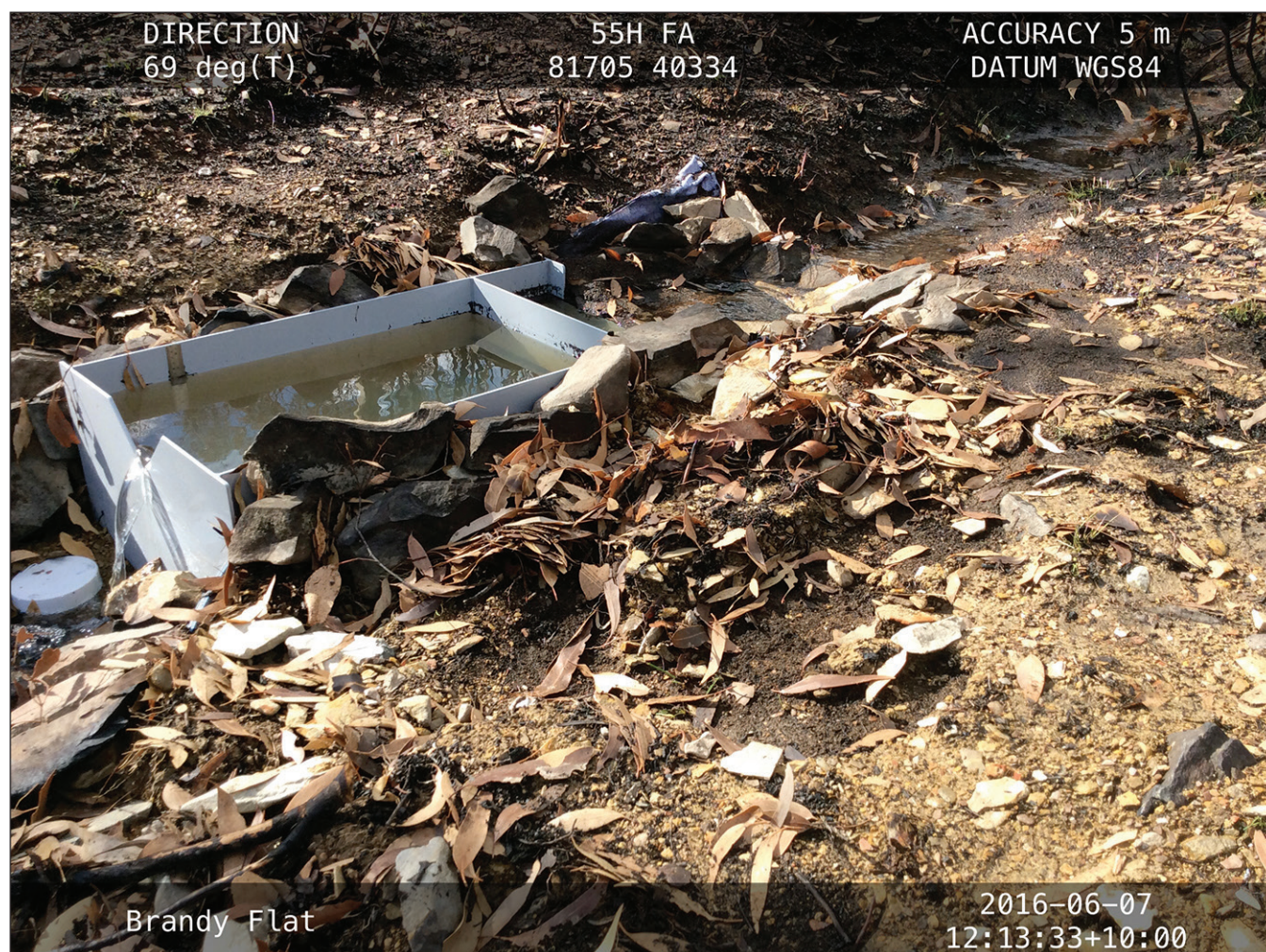
Figure 2 —A sediment trap and a V-notch weir installed in a burned gully.
