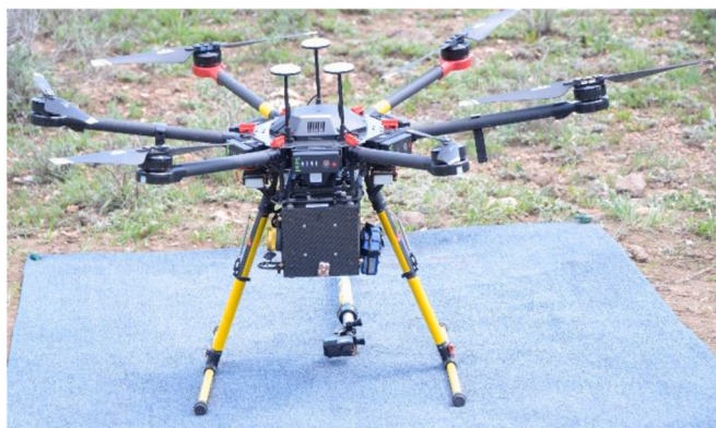
Fig. 1. Kolibri attached to the undercarriage of the UAS.
