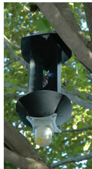
Figure 5.—A panel intercept trap is used to survey for Asian longhorned beetles. Note the packets in the center, which contain lures. When beetles encounter the trap, they are unable to hold onto the black plastic and fall into the collection cup at the bottom. The cup is typically filled with a salt solution or with propylene glycol (antifreeze). USDA Forest Service photo by Melody Keena.
