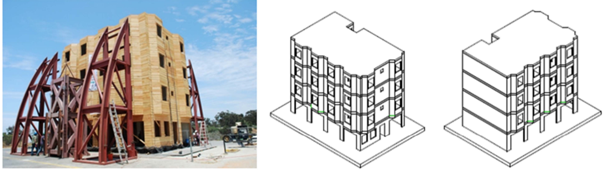
Figure 6. Completed 4-story 4000 sq ft soft-story building ready for shake table testing
