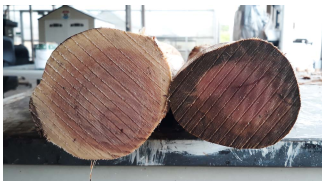
Figure 2.—Healthy (left) and C. lukuohia -infested (right) wood from DOT penetration assays. The dark staining on the diseased bolt is associated with C. lukuohia colonization.
