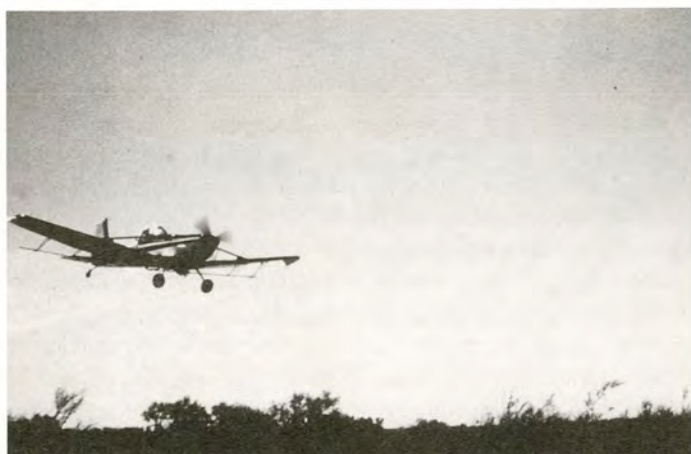
FIGURE 7. Fixed-wing aircraft for applying herbicides. Photo courtesy of R. Bovey, USDA, ARS, Dep. of Rangeland Ecology and Management, Texas A&M University, College Station.
