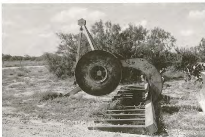
FIGURE 5. A root rake used to remove roots and debris following root plowing.
