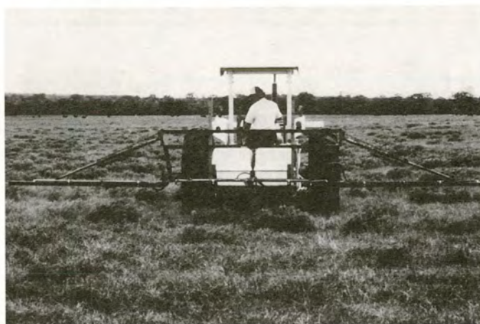
FIGURE 9. Tractor-mounted boom sprayer. Photo courtesy of T. Welch, Texas Agricultural Extension Service, Texas A&M University, College Station.
