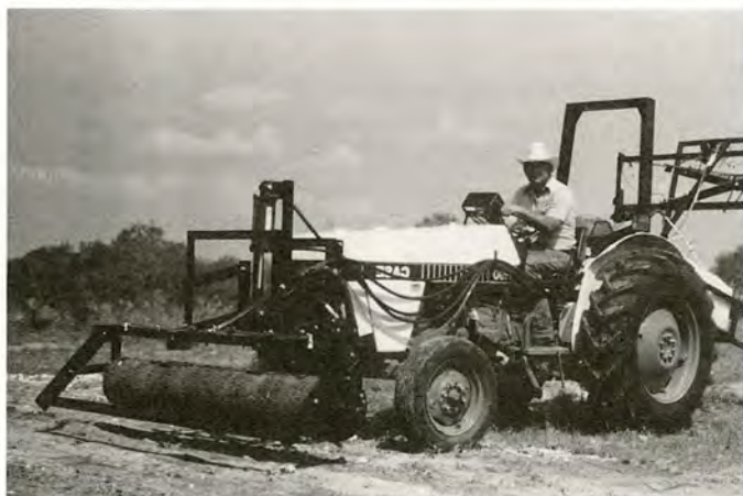
FIGURE 11. Experimental carpeted-roller applicator for herbicides. Photo courtesy of La Copita Research Area, Texas Agricultural Experiment Station, Alice.
