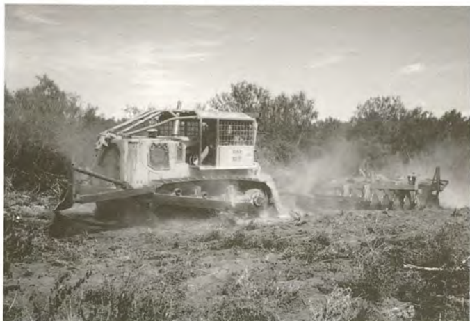
FIGURE 8. Disc plow pulled by crawler tractor being used to manage thornscrub in southern Texas.
