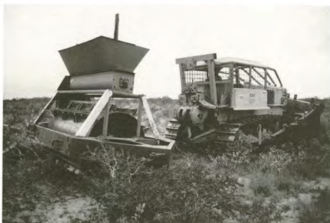
FIGURE 2. Roller chopper pulled by a crawler tractor in thornscrub in southern Texas. A seeder box attachment is mounted above the roller chopper.
