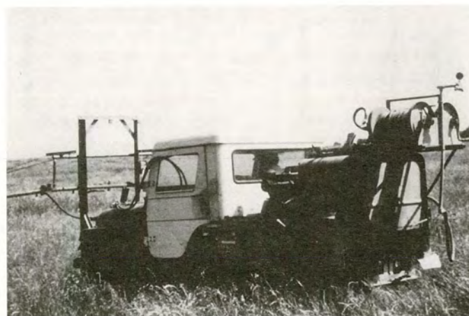
FIGURE 10. Boom sprayer mounted on a 4-wheel drive vehicle. Photo courtesy of T. Welch, Texas Agricultural Extension Service, Texas A&M University, College Station.
