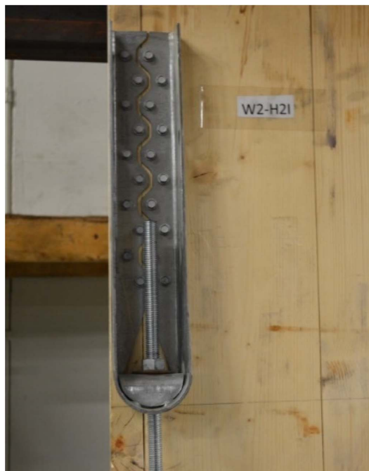
Fig. 20. Simpson Strong-Tie HDU8 hold-down with 15.9 mm (5/8 in.) A36 rod.
