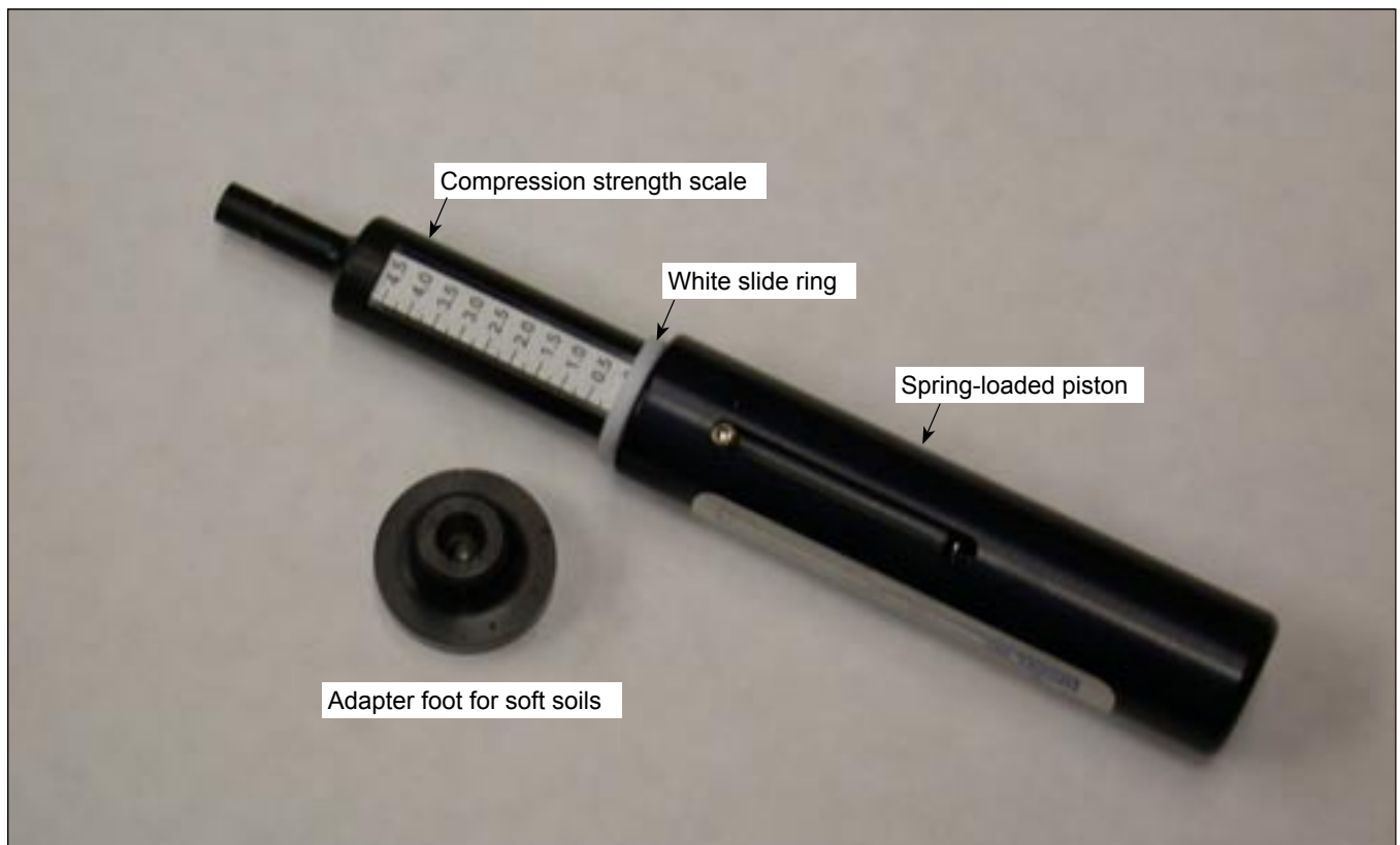
Figure 2. Photograph of the pocket penetrometer and adapter foot.
