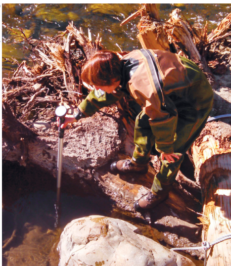
Shannon Claeson measures water velocity on the Entiat River as part of her research with Carlos Polivka on the effectiveness of human-made logjams in enhancing salmon and steelhead habitat.
