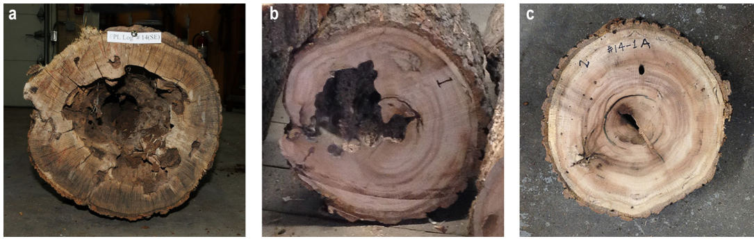
Figure 3: Defects located in the end face and the dissected cross-section of log no.14: (a) void in the end face; (b) rot and void in the cross-section; (c) rot and ring shake in the cross-section.
