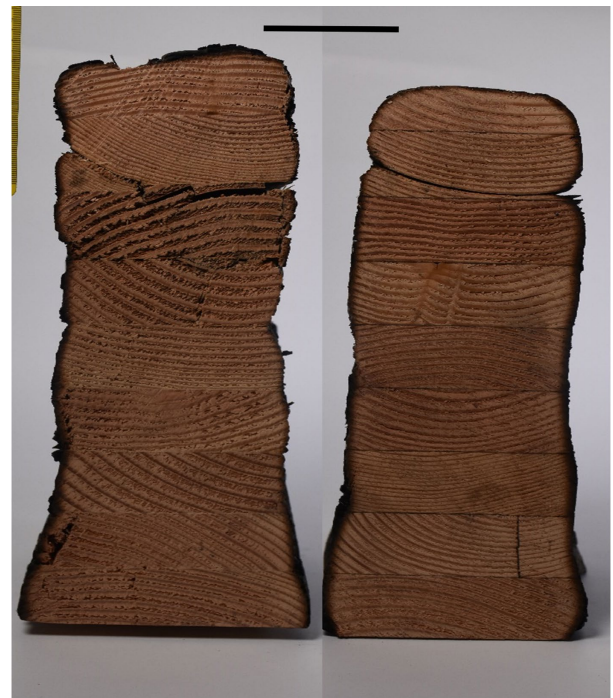
Figure 4. Cross-sectional area at the end of the test for a glulam beam made with an experimental adhesive (left) and a phenol-resorcinol-formaldehyde (PRF) adhesive (right). The scale bar (top of image) is 50 mm long.
