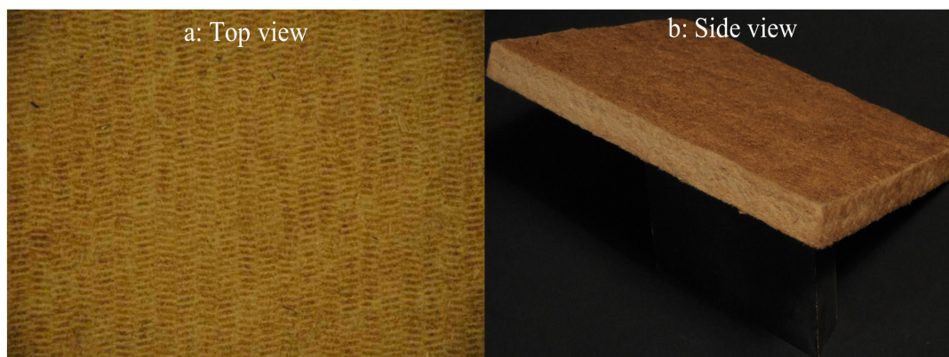
Figure 3. Uncoated cellulosic fiberboard: (a) top view and (b) side view.
