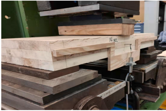
Fig. 6. Short-span three-point bending test setup.
