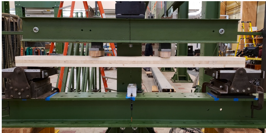
Fig. 3. The test setup for conducting third point bending test with a third-point loading method.
