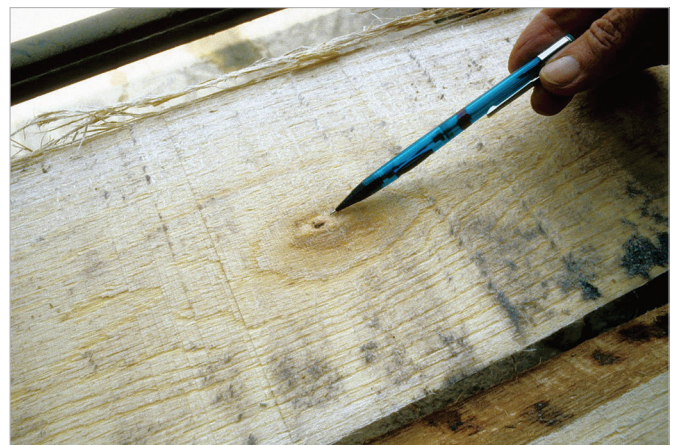
Figure 17 —Epicormic branch defect on willow oak lumber. (USDA Forest Service photo by James S. Meadows).
