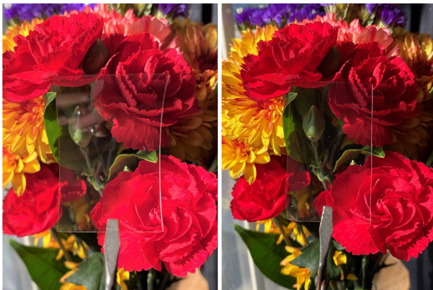
Fig. 1 Photograph show the transparency of TOCNF + 15 wt% PVA composites (left) and TOCNF + 15 wt% PEOX composite (right)
