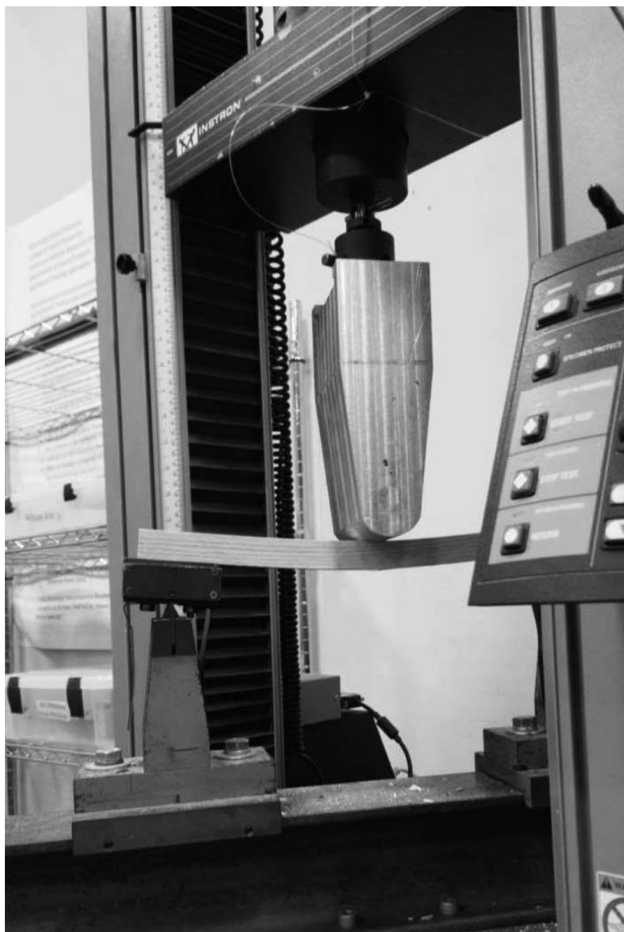
Figure 2.—Center point bending test setup (Sample 3).
