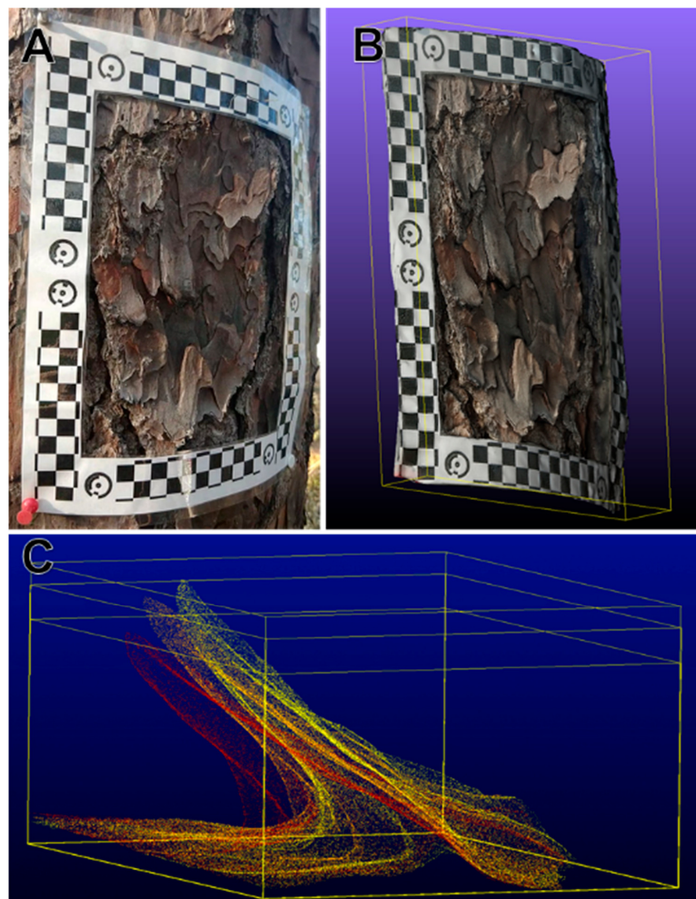
Figure 1. (A) Many individual images of longleaf bark inside a custom scaling frame were processed in photogrammetry software to produce a (B) three-dimensional model that can be sampled and analyzed. (C) A single bark flake cropped from a model tracked through a single day, red at 0800, orange at 1100, and yellow at 1400. The bounding box heights represent the bark flake apex distances from the bark surface that peels away through each time period.
