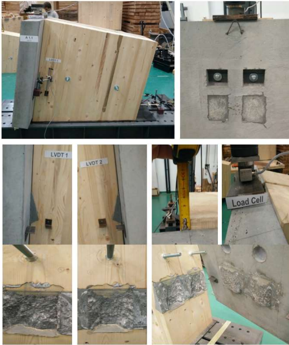
Figure 11: Test specimen (before and after failure)
