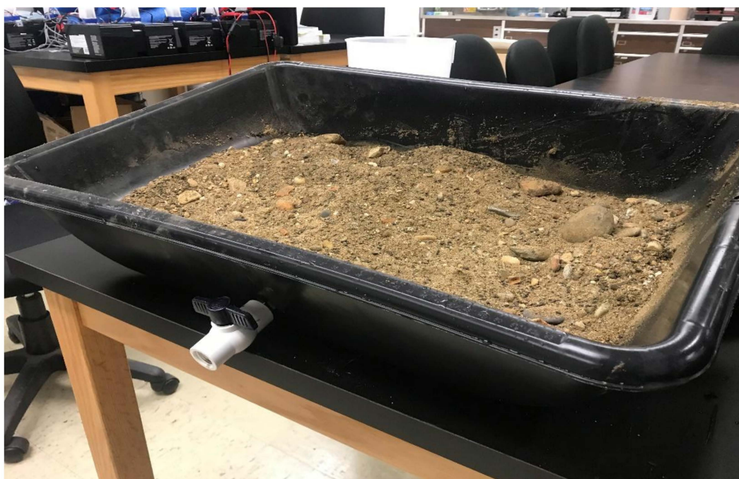
Figure 4. Sediment mesocosm tray set at 10° incline, filled with 6.5 L of hydraulic mine debris collected from the incised creek bed at Blue Point Mine.
