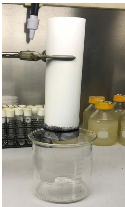
Figure 3. Column set-up is held vertically with a ring clamp and a graduated beaker is placed underneath for collection of flow through. Column contains washed decomposed granite, 0%, 2%, or 5% biochar and 1 L storm water sample collected from Malakoff Diggins. Samples were passed through gravimetrically, and collected in 1 L graduated beaker.
