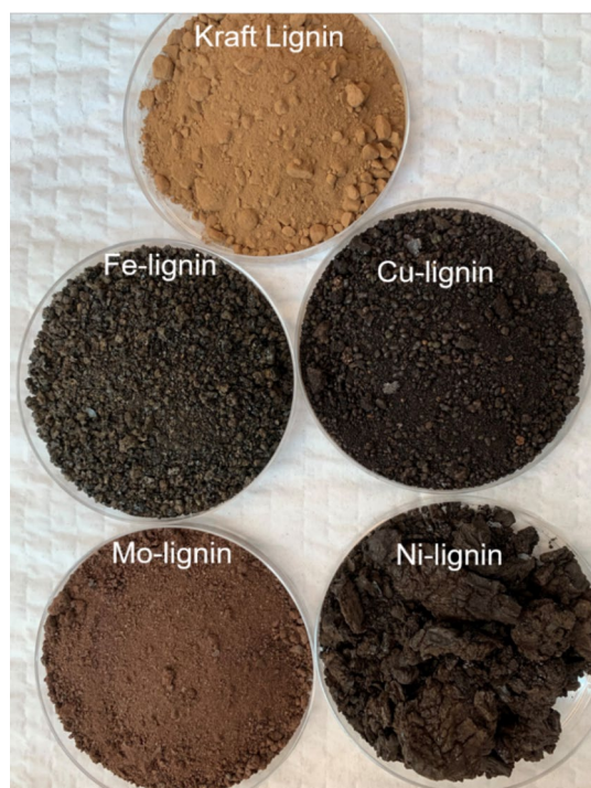
Fig. 3 Physical appearance of Kraft lignin, and Mo-lignin, Ni-lignin, Cu-lignin, and Fe-lignin composites. (Reaction conditions: start temperature, 45 °C; metal content, 10 wt%; salt solvent, DI water; lignin solvent, tetrahydrofuran)
