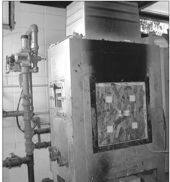
Figure 1—Small vertical furnace at FPL with rim board test specimen.
