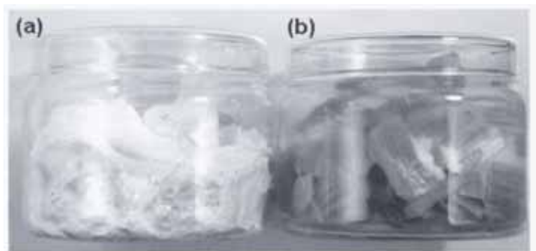
Figure 1. – Mycelial growth of Griofola frondosa on SYP chips: (a) chips treated with extractive-degrading fungi; (b) untreated chips.
