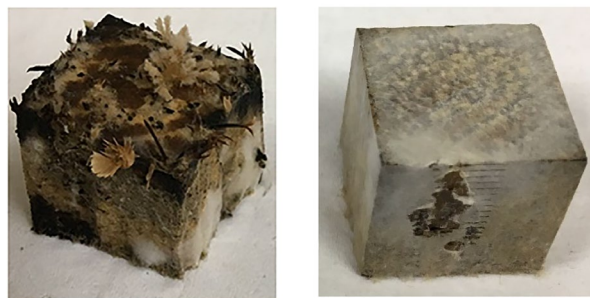
Figure 1. Example image of decay caused by Gloeophyllum trabeum MAD-617 on unmodified balsam fir specimen (left) compared with a specimen thermally modified at 180 °C (right).
