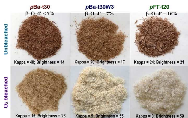
Figure 7. Effect of lignin condensation on oxygen bleaching of WIS from AHF using p -TsOH at 60 wt% and 90 °C. Top row: unbleached WISs. Bottom row: oxygen-bleached WISs at O 2 pressure of 0.75 MPa, NaOH charge of 6% on WIS, and 110 °C for 60 min. Left column: water-washed WIS pBa-t30 from batch AHF for 30 min. Middle column: pBa-t30 washed with p -TsOH three times. Right column: only water-washed WIS pFT-t20 from flow-through AHF for 20 min. Reprinted with permission from ref. [66]. Copyright 2020, American Chemical Society.
