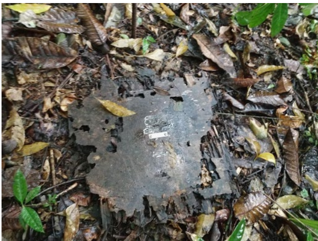
Figure 4— Plywood panel badly damaged by termite attack at Horoko Site, Panama. These untreated poplar plywood panels with MTU-CFRES-WPG tag have been in ground contact for approximately 8 months. Ground and arboreal termite nests were prevalent in this area and indicate very high termite pressure.
