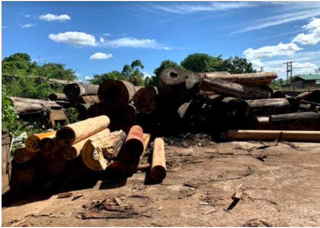
Figure 12—The corner of the log yard of the plywood manufacturer. Heart rot causes problems for veneer production.
