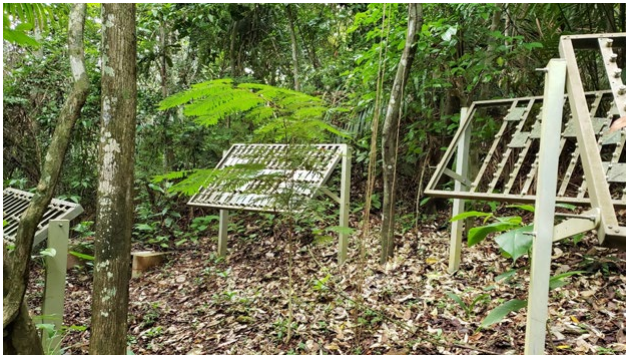
Figure 3— Experimental test racks at Horoko Test Site, originally used for fabric and metal coupon testing, could easily be retrofitted for wood specimens or engineered wood panels.
