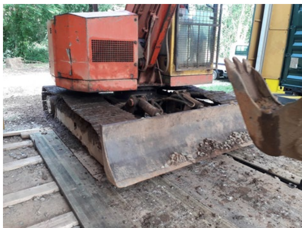
Figure 1—Cyclic abrasion testing with steel tracked excavator on test platforms (photo from TRTC).
