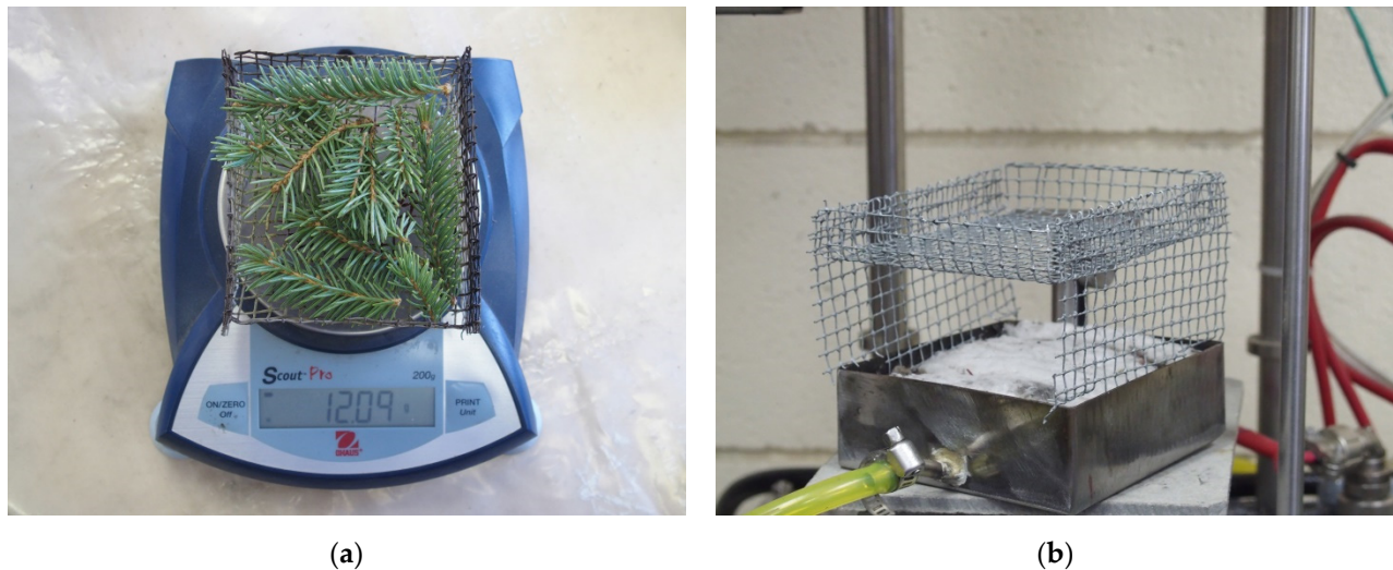
Figure 3. (a) Fuel sample (new shoots) in a 10 × 10 × 1 cm wire mesh sample holder placed on the weight scale. (b) Side view of the empty sample holder. The design of the sample holder provided a constant distance from the shoots to the ignition source and spatial uniformity (constant dimensions and controlled density) of the fuel sample.
