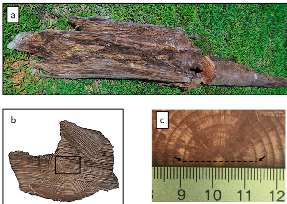
Fig. 1. Southern yellow pine tree section unearthed at The Joseph Pines Preserve in Sussex County Virginia: a) initial cut, b) cross section with rectangle indicating pith and second annual ring zone of interest, and c) closer view of pith with arrows indicating second annual ring diameter measurement.
