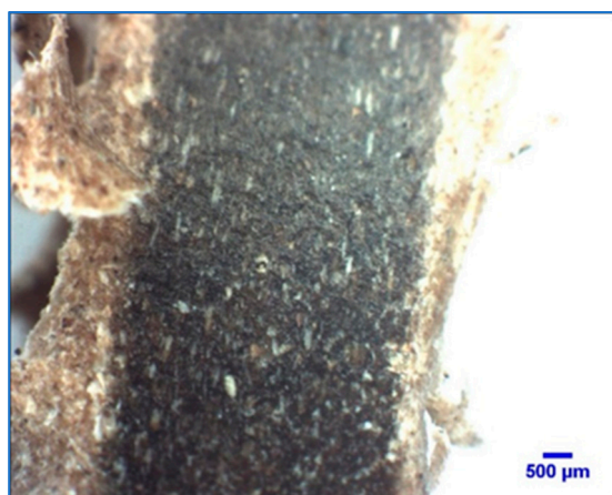
Figure 4. Machined sample of 60 Mesh (40% weight) shows composite mix.
