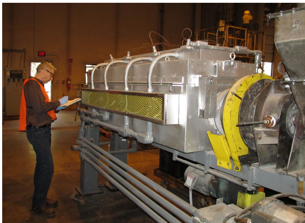
Figure 2. The calciner used in this study shown with one of the authors for scale. Biochar was fed from the hopper on the right into the inlet of the calciner and then moved down the rotating tube from right to left, moving through four heating zones. Photo credit: N. Anderson.
