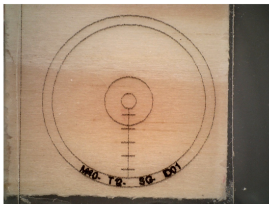
Fig. 4. Specimen target, labelled with MC, Temp, Type, and ID Number. In increasing size, the inner to outermost rings represent 1 mm 2 , 10 mm 2 , and 100 mm 2 in area; the vertical bars are in units of 1 mm lengths.
