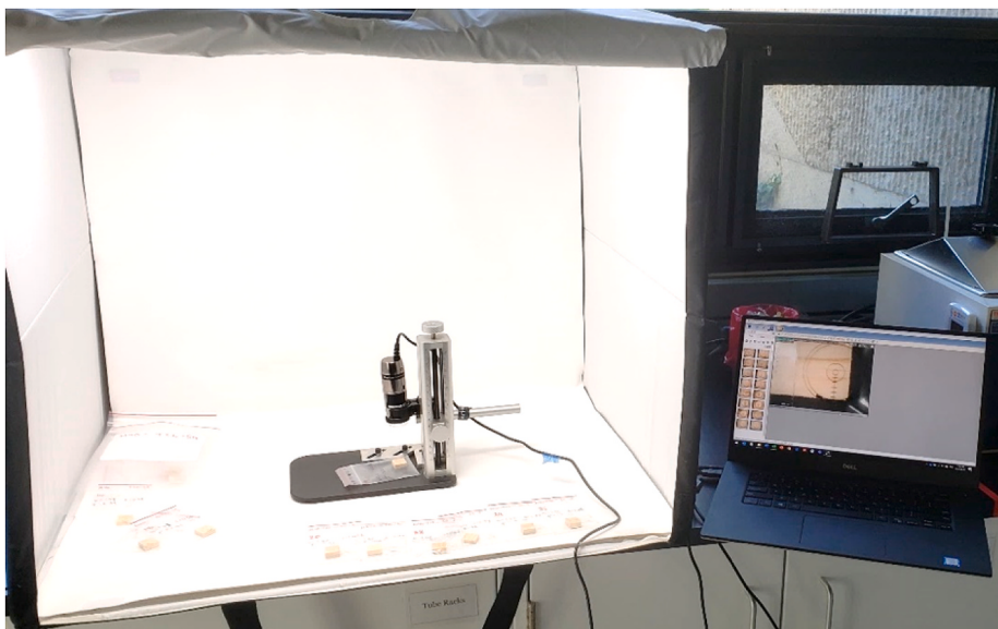
Fig. 3. Photo documentation set-up, with USB microscope showing individually sealed specimens.
